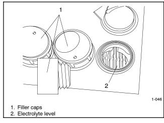
Figure 3-19 Battery Electrolyte Level Inspection
